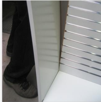
8. While one person holds central panel steady the other person places end panel
